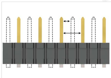
Selectively loading contacts achieves specific creepage and clearance requirements. Contact [asp@samtec.com](mailto:asp@samtec.com)
