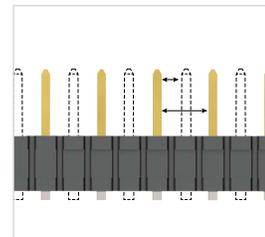
Selectively loading contacts achieves customer specific creepage and clearance requirements. Contact [asp@samtec.com](mailto:asp@samtec.com)
